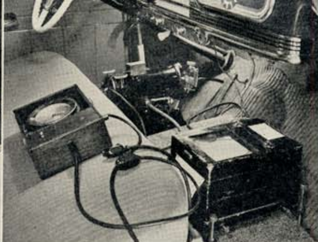
• Mounted behind the fifth wheel speedometer, the little black box precisely measures the stopping distances in the hundreds of braking tests. Right:—The chronometer (on the seat) times the brake machine (rear) powered by compressed air as it depresses the brake pedal exactly at the pressure desired. The recorder (right) marks on tape deceleration time, pedal pressure and pedal travel required to stop the car.
