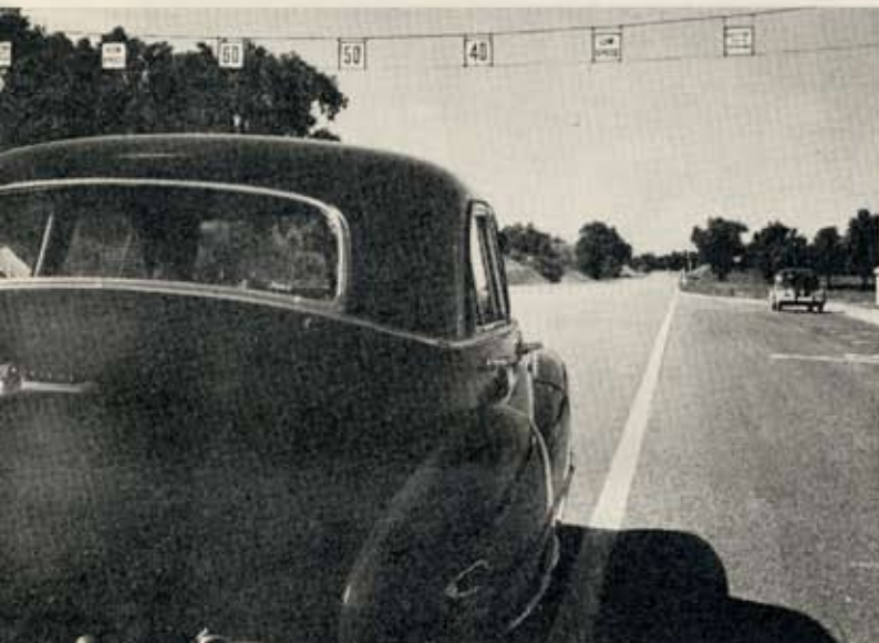
• This straightaway has separate lanes from "Low Speed" to "Wide Open", for economy and durability testing.
