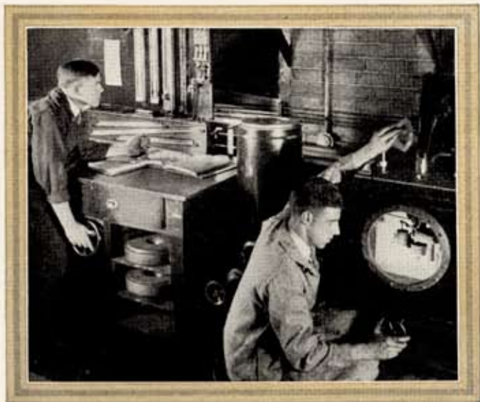
Exact information on a carburetor: Will it start a car easily? Will it feed just the right amount of fuel to the engine? Road tests are not the only answer, for the engineers also determine carburetor performance by putting a carburetor in a mercury sealed box and taking data from precise instruments
