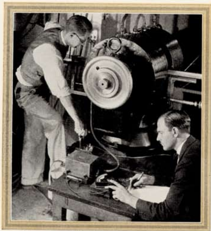
A huge magnet reveals flaws hidden beneath the surface of steel bars. Defects in metal are registered on a meter as changes in electric current
