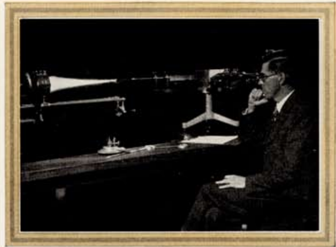
Just as raindrops separate sunlight into the colors of the rainbow, so the spectroscope separates light, from hot metallic vapors, into its component colors. The spectroscope is used in the laboratories to detect minute quantities of impurities in materials, which are unmistakably seen through the eyepiece as a series of bright lines
