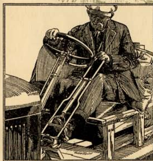
Measuring clutch pedal pressure
