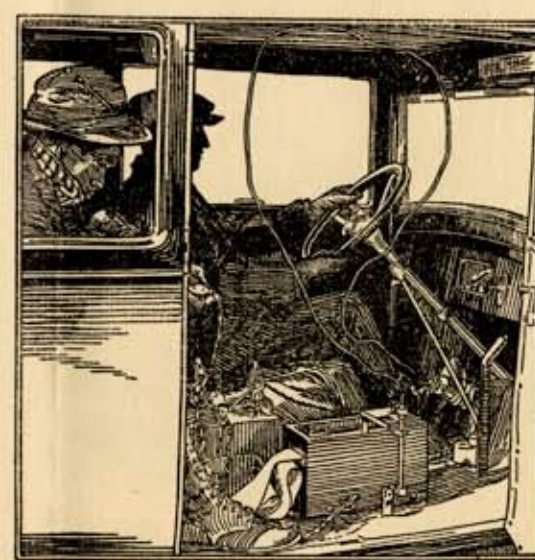
Measuring brake pedal pressure and deceleration
